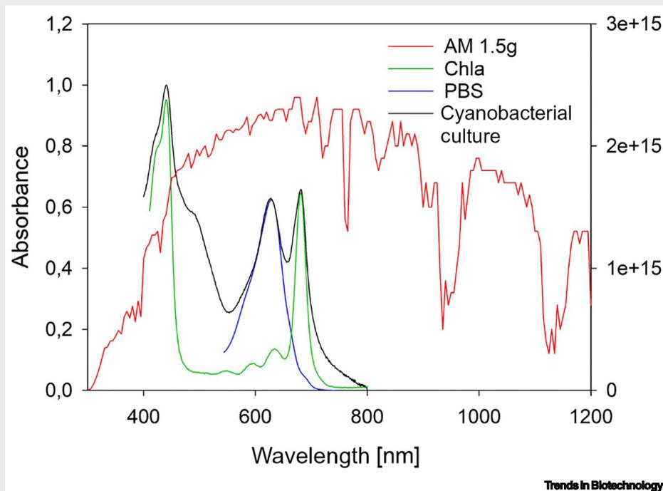
Figure I. The standard solar spectrum AM 1.5g at a zenith angle of 48.5° that is used to determine the efficiency of photovoltaic devices and the absorption spectra of chlorophyll a, the cyanobacterial phycobilisome (PBS) and a cyanobacterial culture. These spectra have been used for the calculation of potential efficiencies above.
